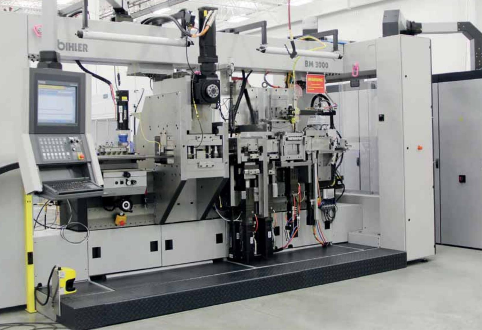
“ Bihler technology is recognized worldwide as a leading manufacturing process for stamped and formed parts from metallic and nonmetallic strips and wires. A further benefit of the Bihler technology is that plastics and other components can be assembled to stamped and formed parts to produce a complete module which provides high added value for the user. ”
