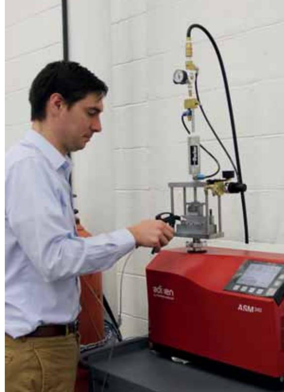
*SUPERB engineer performs a helium leak test on an engineered component with a  $1 \times 10^{-7}$  mbar liters/second leak specification.*
