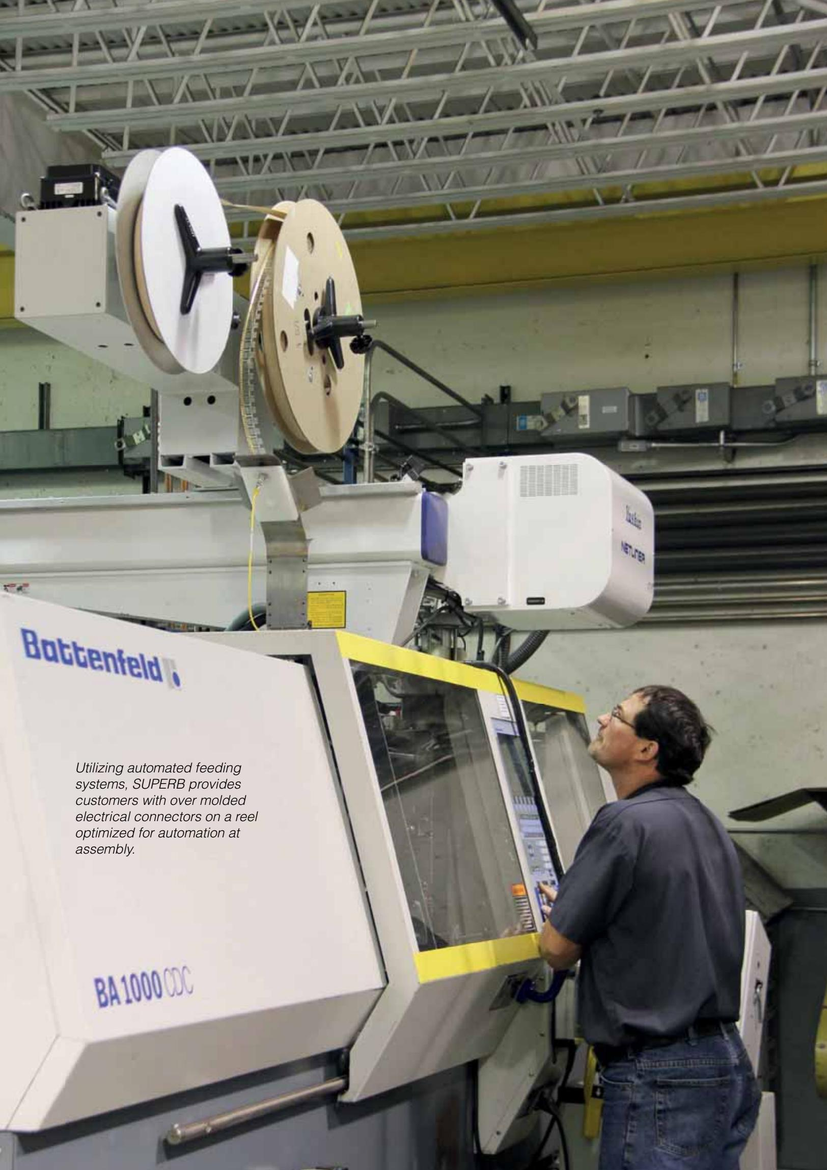
*Utilizing automated feeding systems, SUPERB provides customers with over molded electrical connectors on a reel optimized for automation at assembly.*
